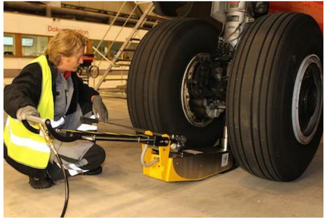
By working closely together with airline operators and production experts, the engineering team at JMS was able to dramatically reduce the component weight for standard axle jacks, improving on maneuverability and ergonomic handling, yet extending the operating speed. Today, JMS counts many of the world's leading airlines as their customer, among them Etihad Airways at Abu Dhabi, relying on J-AXLE products for the time-critical job of wheel and brake changes inside the hanger and on the ramp.
